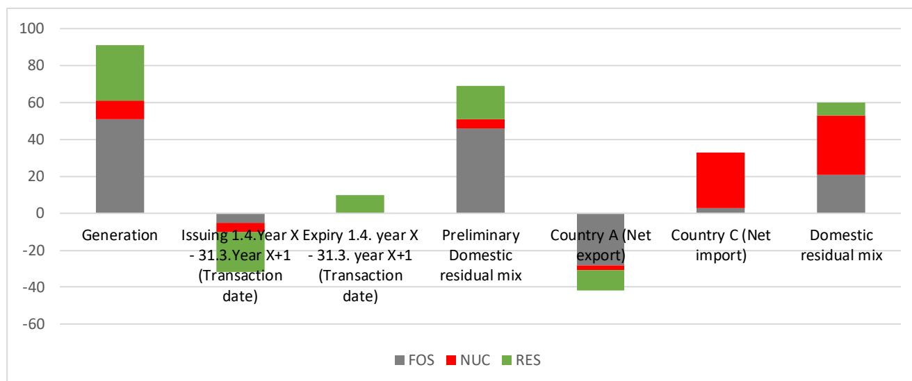
Figure 12: Determining Domestic Residual Mix for countries with electricity exchange across RMC system boundaries. Notice that net export happens with the preliminary Domestic Residual Mix.
